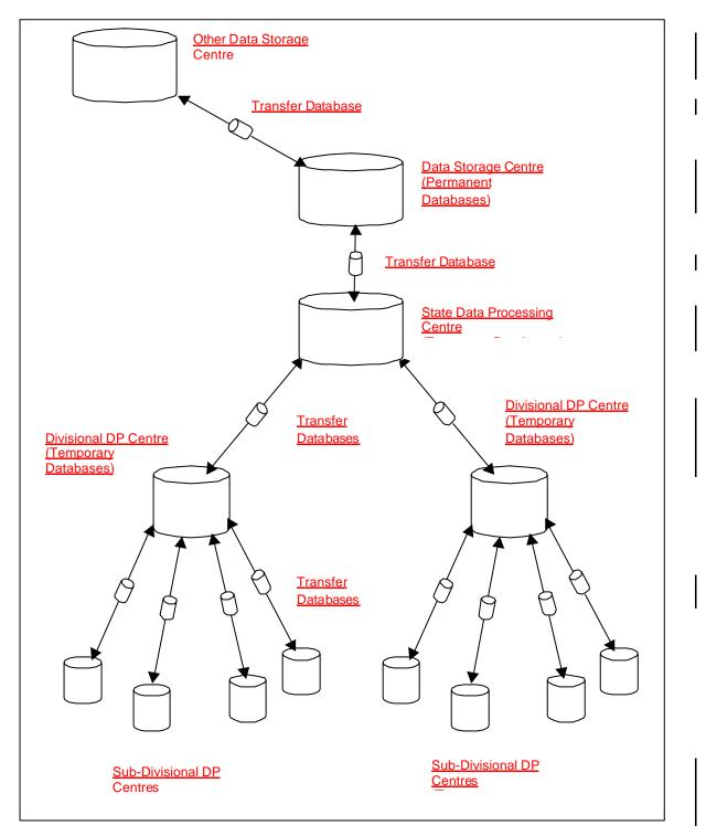
Figure 1.2: Illustration of permanent, temporary and transfer databases
